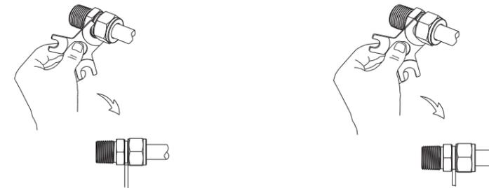
If the gauge can not enter the gap, the fitting is sufficiently tightened.
